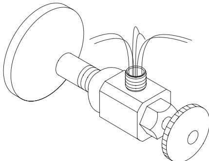
3. Slightly open the main water supply to remove any left over debris.
