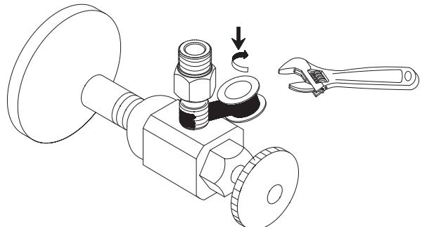
4. Install the special adapter onto the 3/8" supply valves. Apply pipe sealant tape to threads on valve before attaching the adapter.
