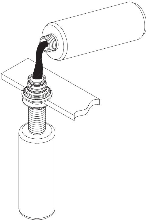
**6. Put the pump nozzle and plastic pump into sleeve.**
