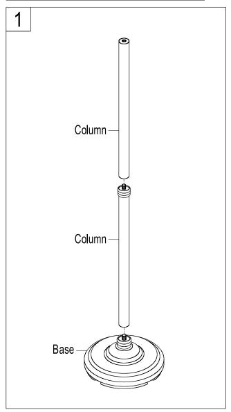
1. Put the base in a level space on ground. Thread one end of column to base in clockwise and connect two columns together.
