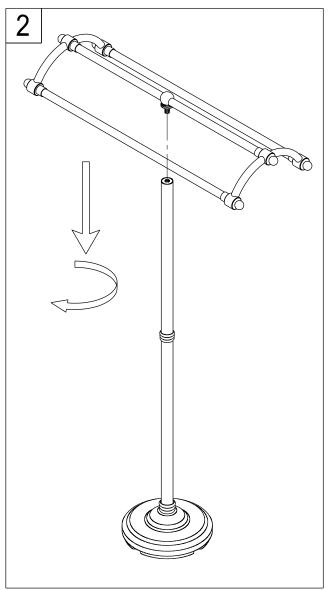
2. Install rack to end of column and hand tighten in clockwise till fully secure.
