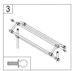
3. Bolt in top rack assembly to bottom assembly.
