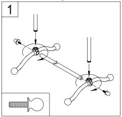
1. Screw in 29" vertical side bars into foot and bolt in bottom bar between assembly.
