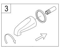
Slide the spout and flange over the pipe. With the spout tight to the wall, tighten the set screw to the pipe.
