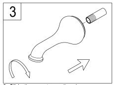
Slide the spout over the pipe. With the spout tight to the wall, tighten the set screw to the pipe.
