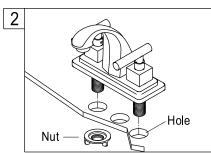
2. Set the faucet in place, insert the inlet shanks through the sink holes, and press down.
