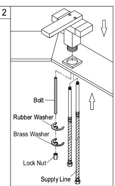
2.Connect the supply lines under the faucet body,make sure it tight so no water will drip. Insert the sprayer hose (bottom end down) through the top opening at the front of faucet body. Use the nut to bolt the faucet onto the counter at the bottom of faucet body. Flange, rubber washer and metal washer should be in place as shown on this diagram. Connect the bottom end of sprayer hose to the opening outlet at the bottom of the faucet body.
