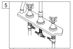
5. Connect the flexible tubes from the supply shank side port to the spout tee. Also reattach the supply lines, turn on the water supply, and check for leaks.
