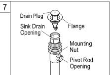
7. Install drain body up through the drain opening and reattach the flange onto drain body, holding the drain body in position with pivot rod opening facing the back of sink, Tighten the mounting nut by hand.
