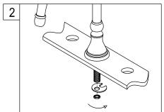
2. Install new faucet spout through the center hole of sink. Place mounting washer on spout shank and attach with spout shank locknut.
