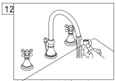
12. Remove the aerator before turning on your new faucet for the first time. Allow both hot and cold water to run for one minute. Replace aerator.
