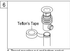
6. Thread mounting nut and bottom gasket onto drain body. Wrap top threaded end of the drain body with teflon's tape.
