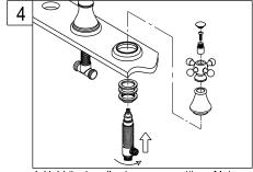
4. Hold the handles in proper position. Make sure that the top of the faucet handles is 5/8" above the top of the sink. Mount the metal washer and locknut from underneath the sink. Than reposition escutcheons as necessary to a desired height.
